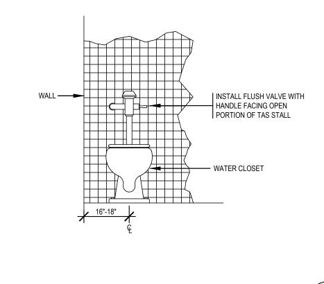
FLOOR MOUNT WATER CLOSET INSTALLATION - TAS NO SCALE
